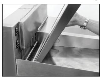
Slide lid until lift flange on lid is under counterweight bar.
